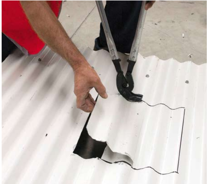
The long arm length of the Metal Pecker allows it to cut through a metal roofing bead or fold, yet is small enough to transport easily.
